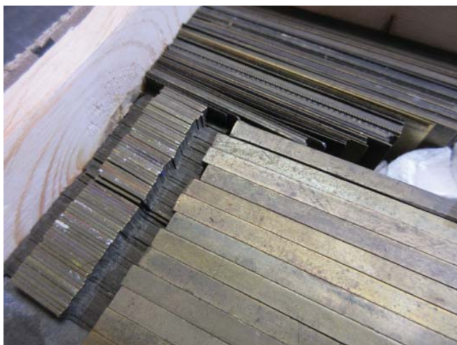
Figure 1. Brass rules in a variety of thicknesses.
